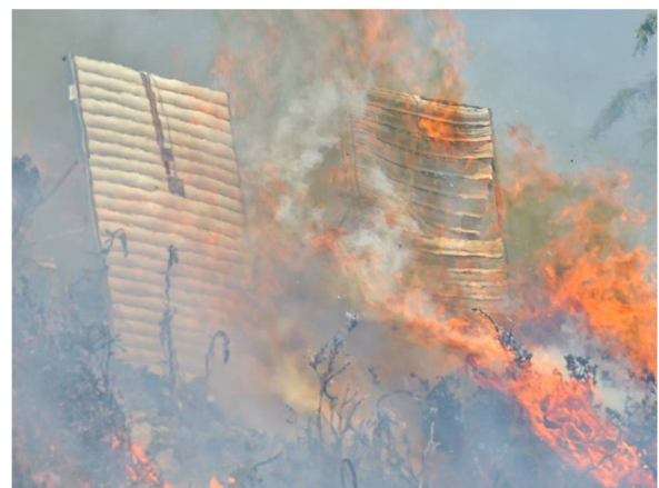
Fig.72. Experimental burnings in Portugal exposing several types of shutter materials, such as PVC (right) and aluminum (left).
