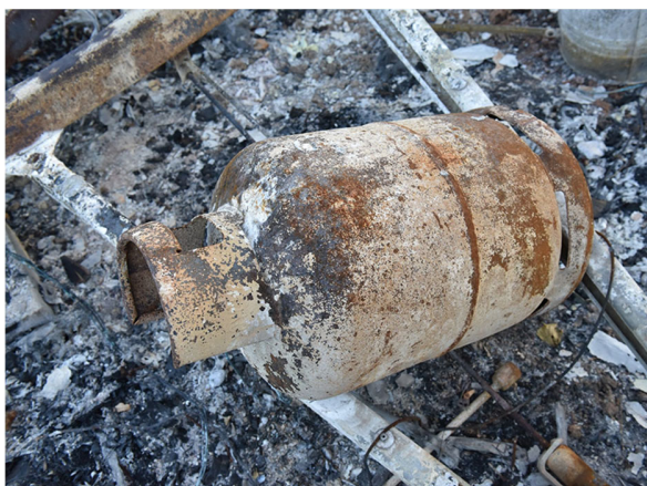
Fig.111. One of the many affected gas canisters in Mati, Greece (2018). Explosions were frequently reported.
