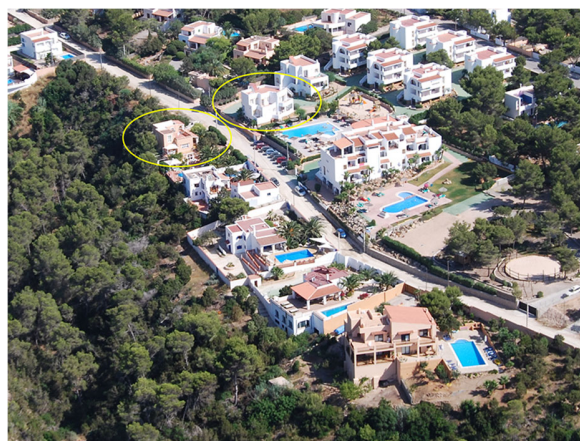
Fig.59. An urban fabric usually provides more protection of buildings located in the interior (centre) than those placed in the border with forested area (left).
