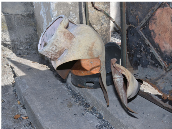
Fig.109. This canister exploded hours after the passage of the fire, when exposed to nearby combustion in Funchal, Portugal (2016).
